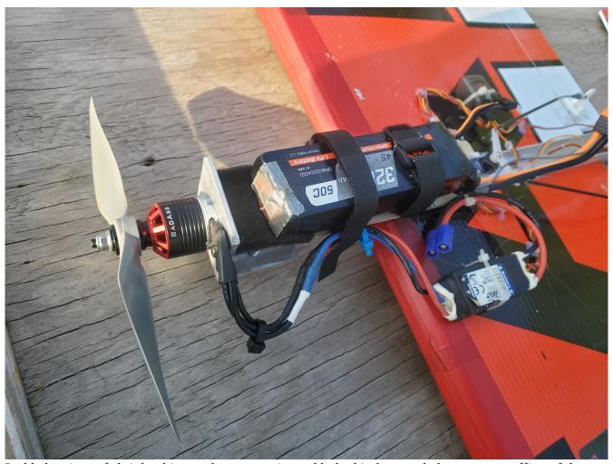
I added a piece of shrink tubing to the motor wire and bolted it down to help prevent scuffing of the wires. Of course, the motor mount could be cut down further too. I strapped the ESC and receiver down along with some Velcro. I actually had the receiver come off mid flight with using just Velcro. It was a hard landing! No damage other than a broken prop.
